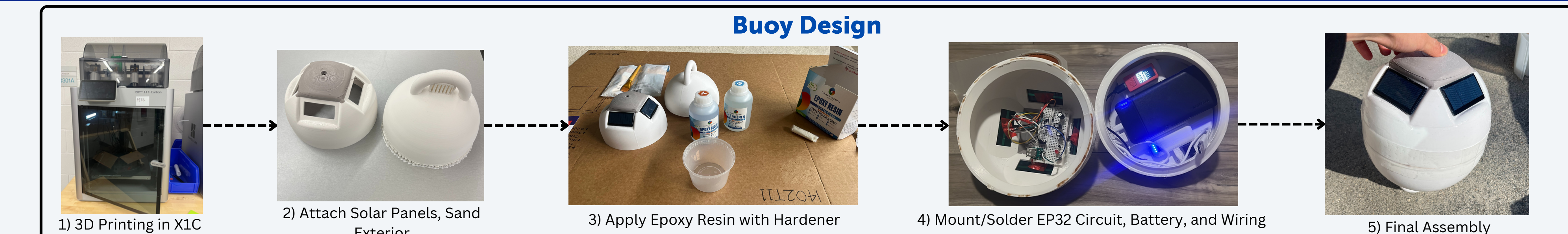
Figure 13. After 3D printing, the buoy was sealed with epoxy resin to ensure waterproofing. Onboard electronics consist of an M5Stick-style ESP32, which in full deployment will interface with an LTE modem and a hydrophone; during benchmark tests, Wi-Fi and a standard microphone were used instead. All components—the ESP32, battery, and solar panels—are wired on a breadboard mounted to the buoy's lid and powered via USB from a dual-battery pack. (All images taken by researchers)
